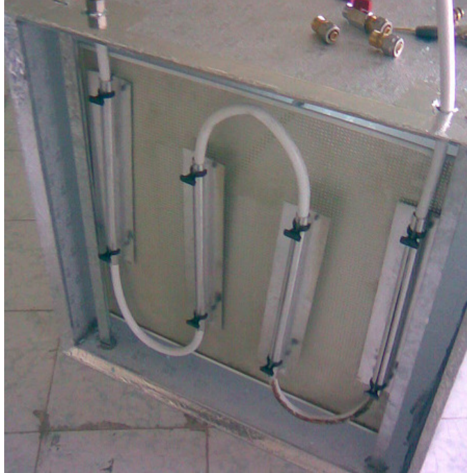
Fig. 4: Thermo pipe with aluminum fins
